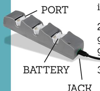
1. Connect the power cable to one end of the charger and plug into wall. Verify green light on charger jack is on.
